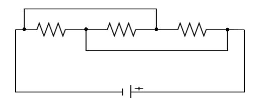
Consider the circuit given below. Each resistor has the same value R and the battery's voltage is V. Find the total current flow through the battery. *The loop in the diagonal wire means that it loops over the other wire and is connected only on its ends.*
