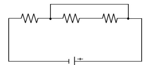
Now, you add one wire to the same circuit as shown. Though there is only one additional wire, there are more paths going from one side of the battery to the other. Find the total current flow through the battery at this time.
