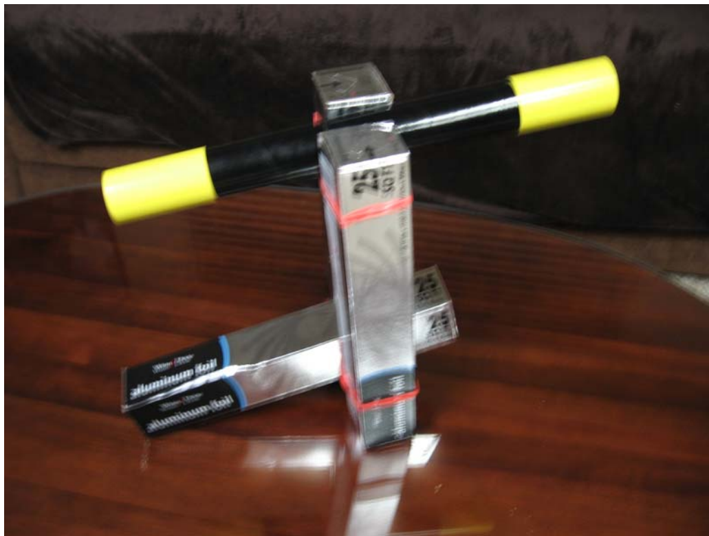
Figure 4: The assembled telescope and foil box mount. This inexpensive mount is very steady.
